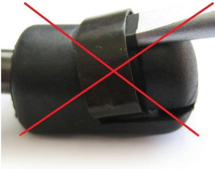
The use of any object aiming to separate or to take off the metal retaining ring may cause the deformation of the ball socket. The ball socket is no longer maintained on the bolt.
