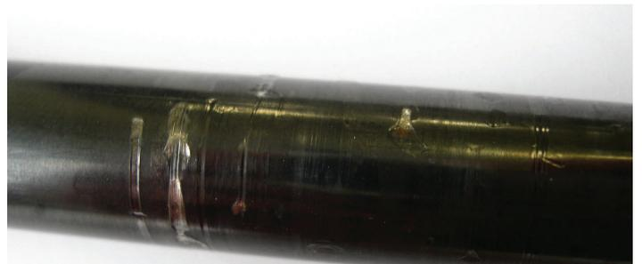
Tightening with a pliers
