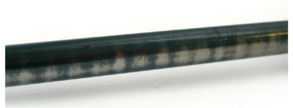
**Solution :** It is necessary to check the alignment, and if you need, change the end-fittings. It is necessary to use a margin of functioning on the axis 0.3 to 05 mm and a margin of functioning on each side of the end-fitting from 0.5 mm to 1mm max.
